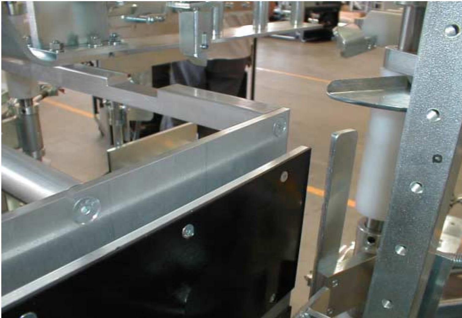
The movement of these paddles is controlled by the cam and linkage located on the right side of the machine.
