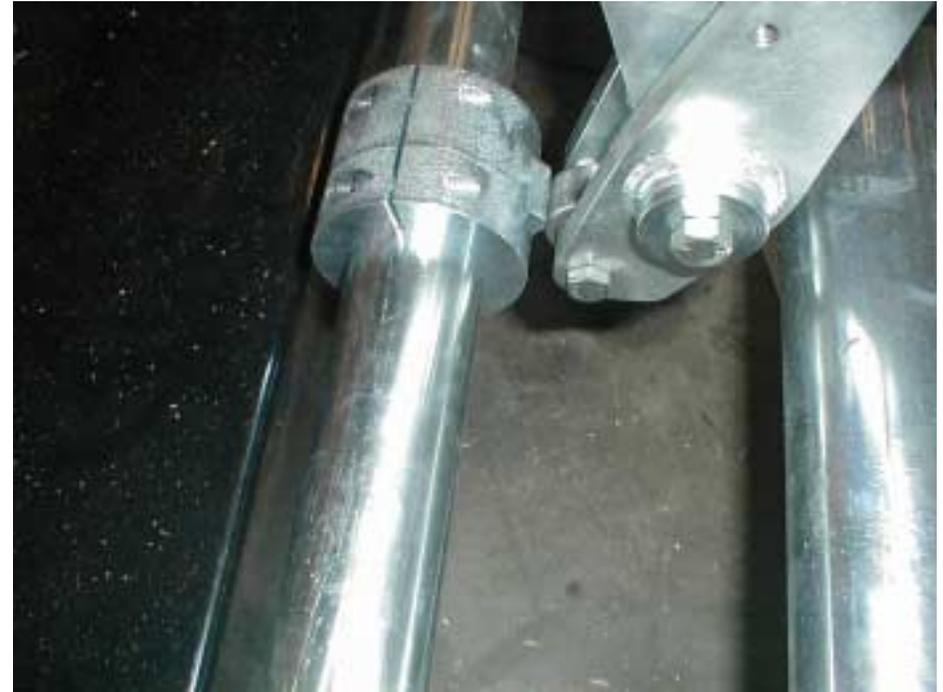
The minor flap breakers are used to pre-break the minor flaps from the main blank as the mandrel is on its forward forming stroke. The arms are operated by the small lobed cam that is located on the right side of the machine. The cam is timed so that it comes up on the high point as the front of the mandrel reaches the center of the vertical trees.
