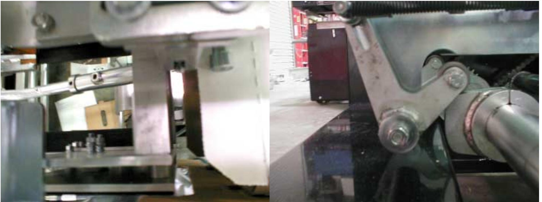
The inside flap folder is operated by the cam the is located on the left side of the machine. The cam is timed so that when the mandrel if on it's back stroke and the front of the mandrel is just clear of the box strippers, at this point the cam is just starting to come up on the high point.
