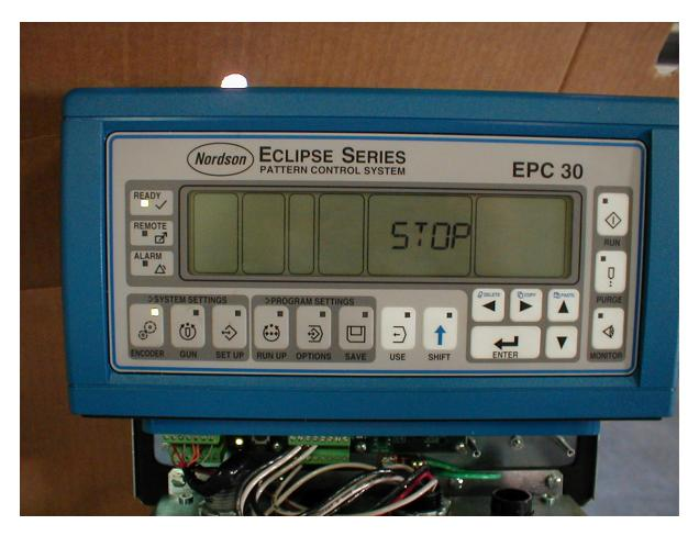
After running the blank past the trigger, the display will change to stop.
