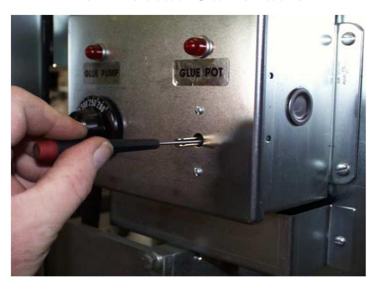
Turn on machine and allow adhesive to reach operating temperature (about 1/2 hour warm up time). Using a surface probe pyrometer, measure the temperature just above one of the glue jets (refer to Figure 7-1 for correct probe location). If the temperature measured with the pyrometer is the same as shown by the thermostat control knob, the thermostat is calibrated. If the temperatures are not the same, recalibration can be accomplished by the following method.
